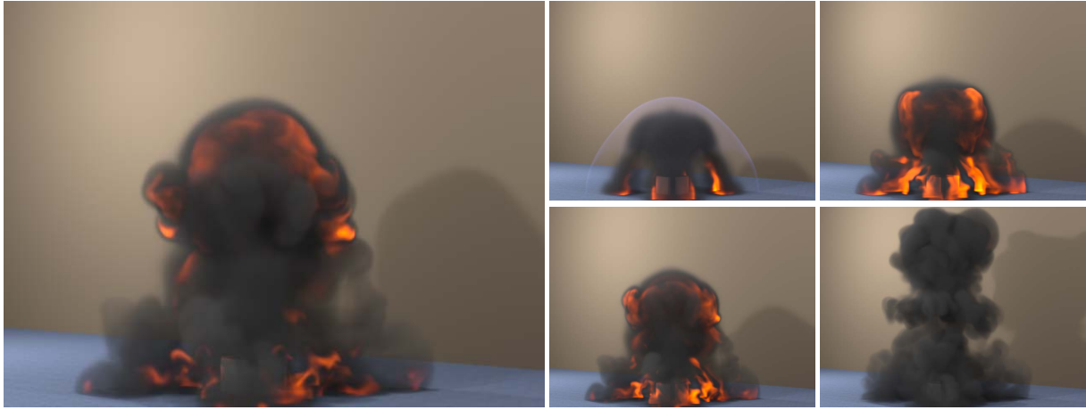
Figure 3: A charge is detonated within a small four-walled chamber at t = 0 . Shown on the left is a smoke plume at t = 0.04s , and on the right its development, at times .005s , .02s , .03s and .115s . This was solved on a 200 \times 300 \times 200 grid.
