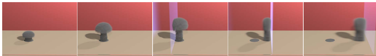
Figure 10: After a smoke plume develops, it is hit by a planar shock. Times shown are .83s, 1.67s, 2.0835s, 2.0836s, 2.0838s. The grid resolution is 512 \times 256 \times 256 .
