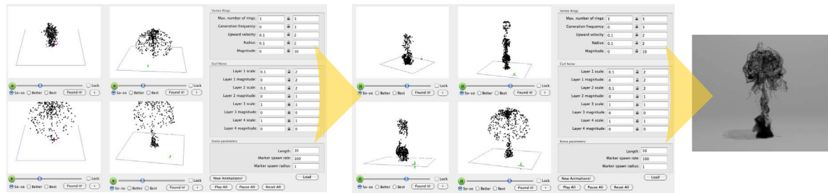
Figure 1: The animation gallery in action. An animator is searching the space of possible parameters to find an animation. He or she provides preferences over a gallery of animations created procedurally from different parameter settings. The system uses these preferences to automatically learn a model of what the user is searching for and to propose a new set of animations. The new gallery automatically balances the exploration-exploitation tradeoff between finding improvements on animations the user likes and exploring new settings. It also incorporates user constraints about what parameters or ranges to search. When acceptable parameters are found, a higher-quality animation can be generated offline. As the tool is used, it automatically learns the properties of the parameter space that generate good animations — the more it is used, the better able it is to guide new users.
