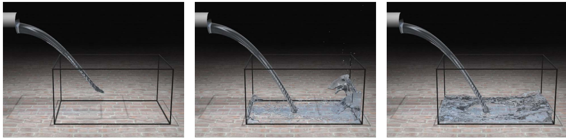
Figure 9: Offline rendered images using POV-Ray of a simulation with 250'000 particles using our CUDA based SPH solution. On average 5.6 physics time steps per second are reached on Platform 1.
