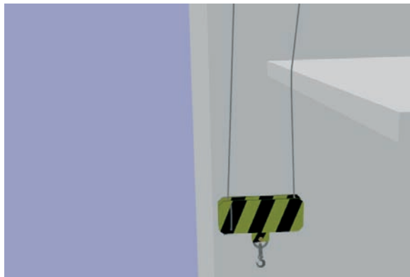
Figure 6: A tower crane cable collision.
