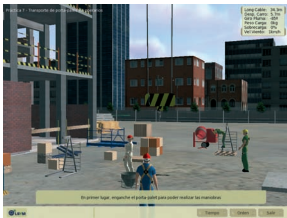
Figure 10: A screen shot of the tower crane simulator developed at University of Valencia.
