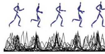
Figure 4: In recorded human motion, local motion features are temporally correlated to changes in movement of the corresponding body parts. When many parts of the body change direction together, many features cluster nearby in time, which appears as greater peak density and height.
