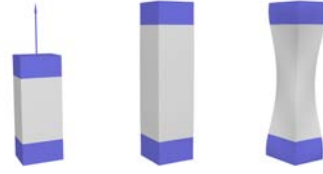
Figure 3: Illustration of the effect of the different shape modeling constraints. Left: handle constraints are specified to fix the bottom of the box and to move the top to the desired position. Middle: with only the rigidity constraint the total volume is increased by 53%. Right: the total volume remains within 3% of the original when the volume constraint is added.
