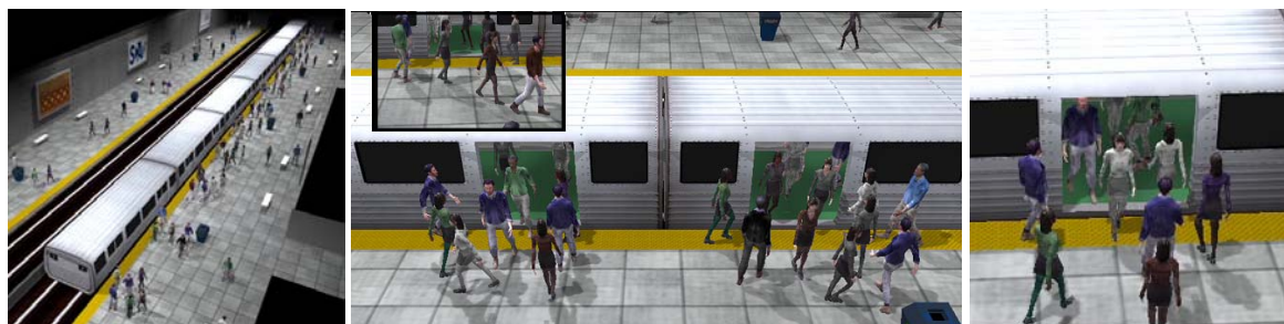
Figure 8: A crowded subway station: The exiting agents have a higher priority and are given preference to pass through the doorway first. The priority proxy formulation eliminates the need for any kind of explicit coordination between the exiting and boarding agents.
