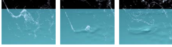
Figure 2: Impact of falling droplets on water surface. The individual masses of the particles are minuscule. However, their impact accumulates as the droplets continue to hit the surface, causing noticeable ripples.
