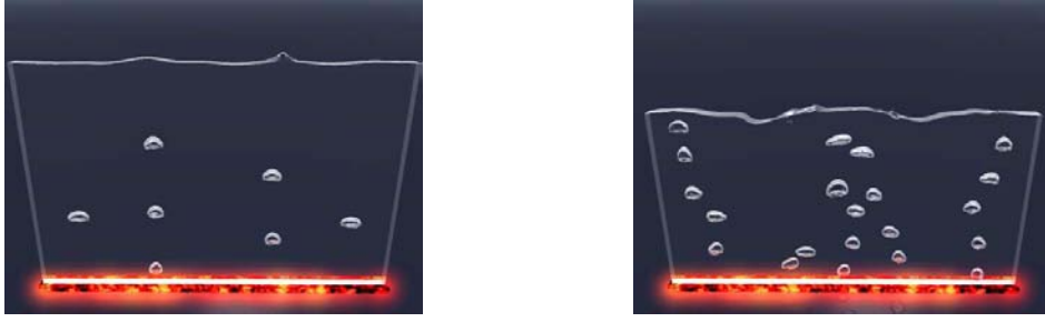
Figure 3: Circulation increase in a boiling flow: (a) early "straight" pattern (b) late development mixing pattern
