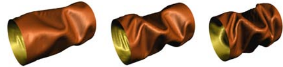
Figure 11: Sequence taken from an animation of axial compression of a sleeve with a metal-like material.
