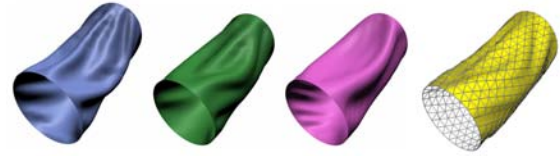
Figure 10: Fabric sleeves under gravitational loading with different material parameters. Right: Mesh used in computation with 494 Vertices and 936 faces.
