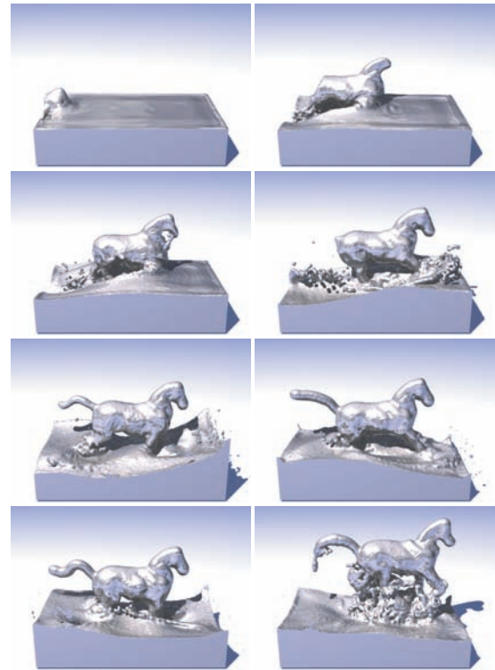
Figure 6: An SPH fluid following the shape of an animated model. Control particles are created by sampling the interior of the horse.
