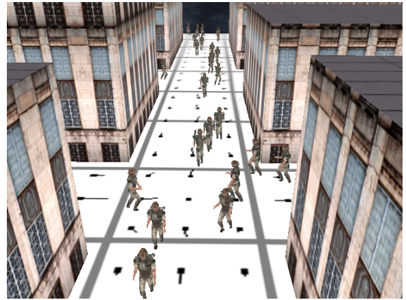
Figure 9: A frame showing people moving through a city, driven by a flow tiling of the streets. Internal boundary conditions prevent people from walking through building walls.
