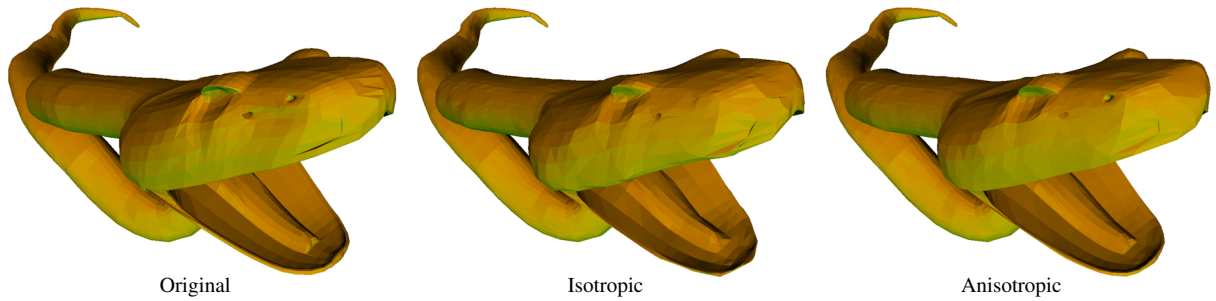
Figure 3: Left to right: original, isotropically compressed, anisotropically compressed meshes of the frame 100 of the snake sequence. Both reconstructed meshes are I-frames compressed at 2 bits per vertex (see Section 4.1). Note that anisotropic version reconstructs both nose holes, and results in a sharper reconstruction of the tongue, as well as the smoother curve of the bottom jaw silhouette.
