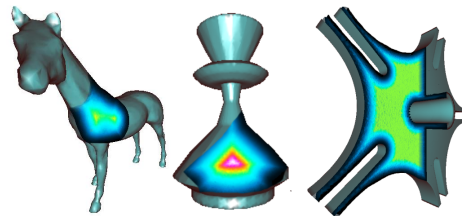
Figure 7: The 3D distance field of large objects (horse, pawn, imprison) compose of 300000 tetrahedrons is computed with CPFM in 0.1s.
