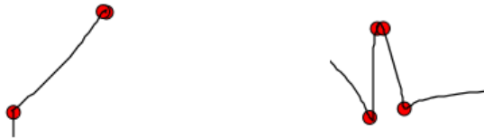
Figure 3: Two example of sharp noise: caused by hook (left) and caused by sharp angle (right).
