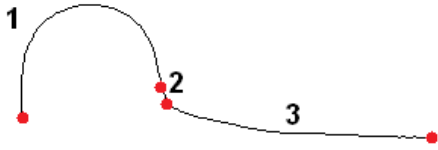
Figure 4: Initial set of corners found for a stroke consisting of an arc and a line. Segment 2 is the smallest, unneeded segment and should be merged with Segment 1.
