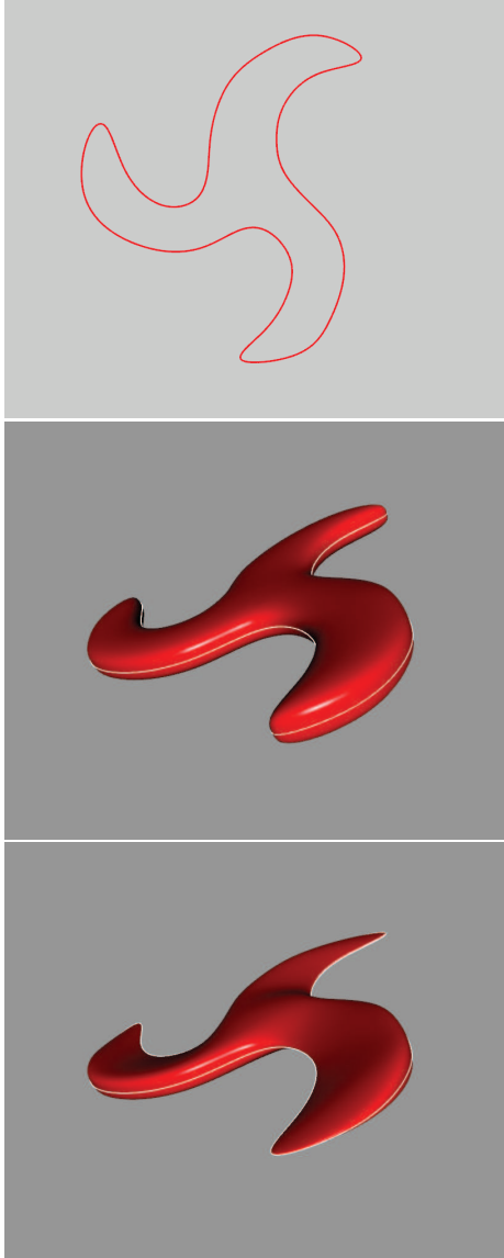
Figure 7: A 3-blad fan without (top) and with sharp features across the profile curves.
