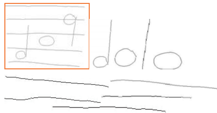
Figure 21: The top left image in red shows the original paper-sketched image, the right images show the extracted strokes after merging.
