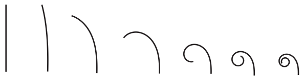
Figure 6: Fixing arc length and an initial curvature parameter, a family of clothoid segments is formed by decreasing parameter B near infinity (left) toward zero (right).
