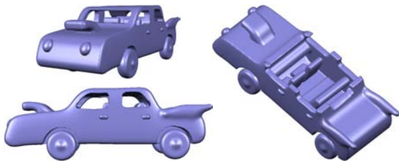
Figure 16: The body of this car model was initially sketched, and then the internal structure was carved out. Right image shows cut-away view.
