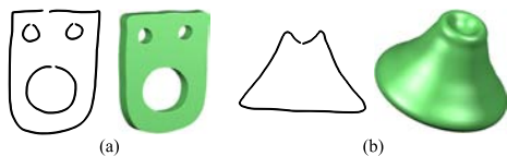
Figure 2: Sketched 2D curves can also be used to create (a) linear sweeps and (b) surfaces of revolution.
