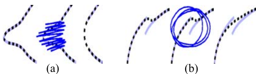
Figure 9: Examples of the eraser gesture (a) and smooth gesture (b). These gestures manipulate the parameters used to compute the final variational curve (dashed line).
