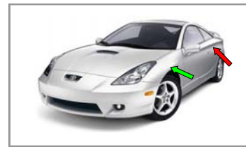
Figure 5: Example of an accent line with change of continuity along itself (the green arrow points to G^1 continuity, while the red one to G^0 continuity) (courtesy of Toyota).
