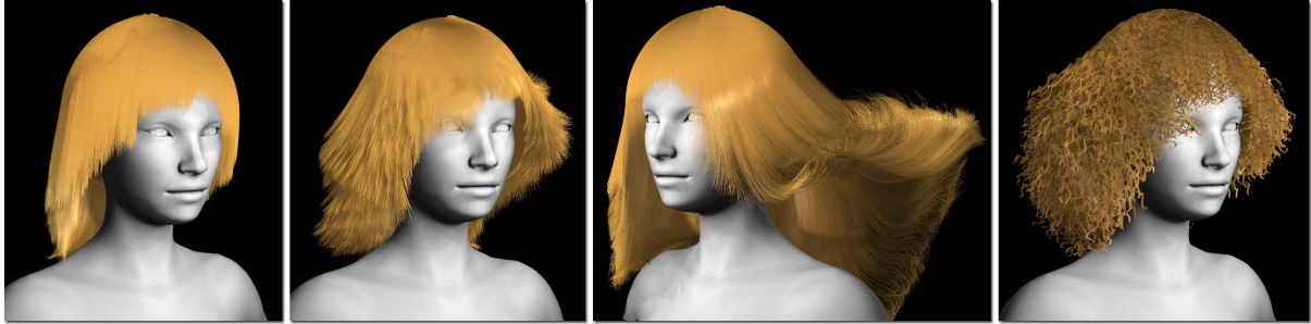
Figure 1: Our method allows the simulation of every hair strand in real time. From left to right: 47k hairs simulated at 25 fps including rendering and hair-hair repulsion. Long hair composed of 1.9m particles at 8 fps. Curly hair using visualization post-processing.
