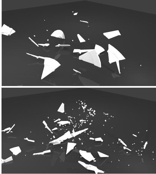
Figure 1: Application of the precomputed shapes method to a plate which is broken through a procedural fracturing process. Each fragment is associated with collision detection and inertia data from the database. A rigid body simulation can then be run.
