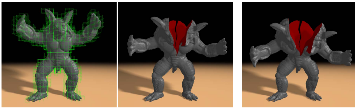
Figure 6: Left: The coarse hexahedral simulation grid and the high-resolution surface that is constructed from the embedded fine grid. Middle: Simulation using composite elements obtained from coarsening the hexahedral finite element model by three levels (10,563 DOFs). Each simulation time step takes 176.37 ms. Right: Simulation of cuts in the Armadillo model using hexahedral finite elements (569,748 DOFs). Each simulation time step takes 2829.87 ms.
