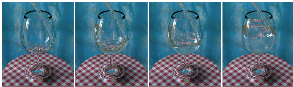
Figure 5: Glass scene. Filling up a glass with up to 75K fluid particles. The whole glass consists of 39K boundary particles. Overall computation time 4 minutes, \Delta t_{min} = 0.0015 , \Delta t_{max} = 0.0022 .
