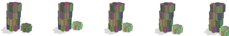
Figure 9: Still frames from an interactive simulation of a medium sized configuration, with approximately 280 contact points yielding 840 variables. The Fischer–Newton method is implemented in Java and uses 6 milliseconds on average per frame. The program utilizes one core on a 2.1 GHz CPU Duo Core.
