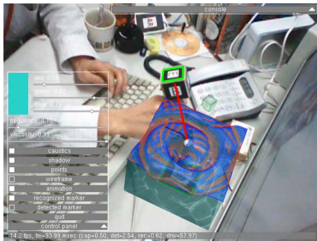
Figure 7: Visualization of acceleration. Red points show upward acceleration and blue points show downward one.
