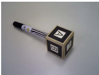
Figure 4: The AR pen: A cube composed of five AR markers is attached at the end of a pen.
