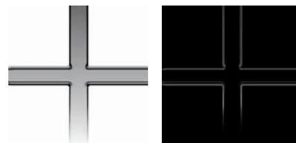
Figure 3: “Simple” image texture: original image and discontinuity map by Sobel filtering.
