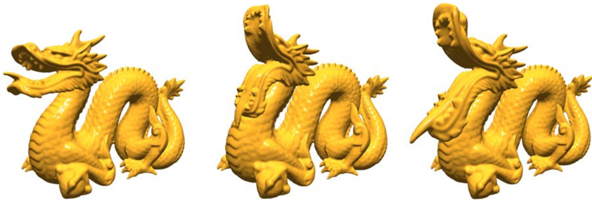
Figure 1: On a desktop PC, the tetrahedral grid consisting of 67k elements (left image) was interactively deformed at 3 tps using the corotational finite element formulation (middle image). Additionally, the same model was deformed using the small-strain formulation at 17 tps (right image). The artificial volume increase of the mouth can easily be perceived.
