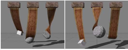
Figure 8: Cloth stripes are attached via one way interaction to static rigid bodies at the top and via two way constraints to rigid bodies at the bottom.
