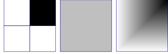
Figure 6: 2D stiffness in level of gray. From left to right: a) four original cells, three empty, one full. b) the corresponding cell with uniform weighted behavior presented in section 5.1. c) the corresponding non-uniform cell presented in section 5.3, stiffness varies along the axes
