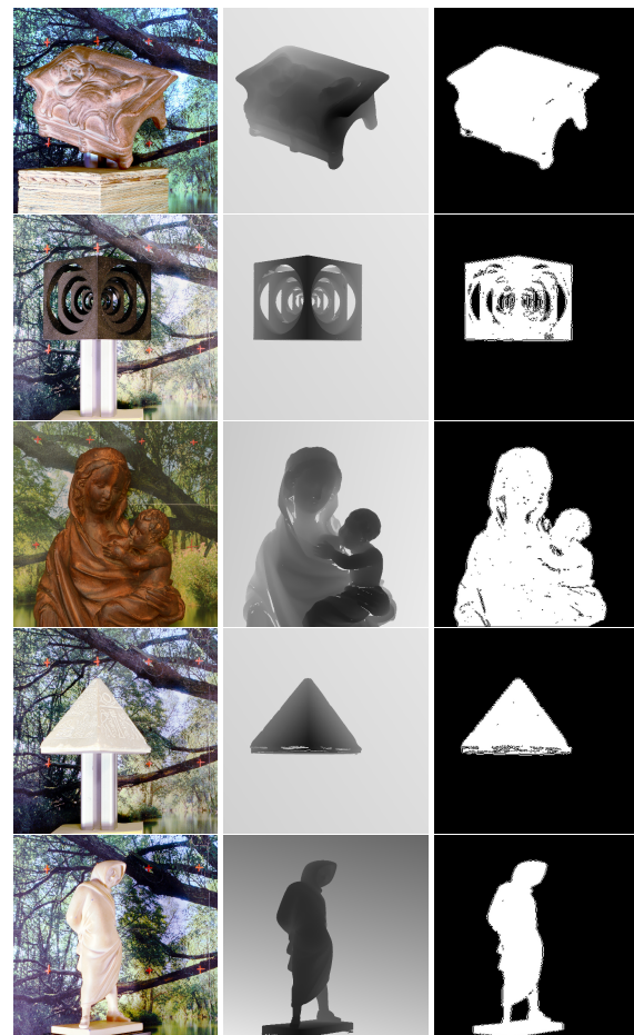
Figure 1: Datasets in the category Gantry. From left to right: center view, depth channel, mask which indicates regions with valid depth information.
