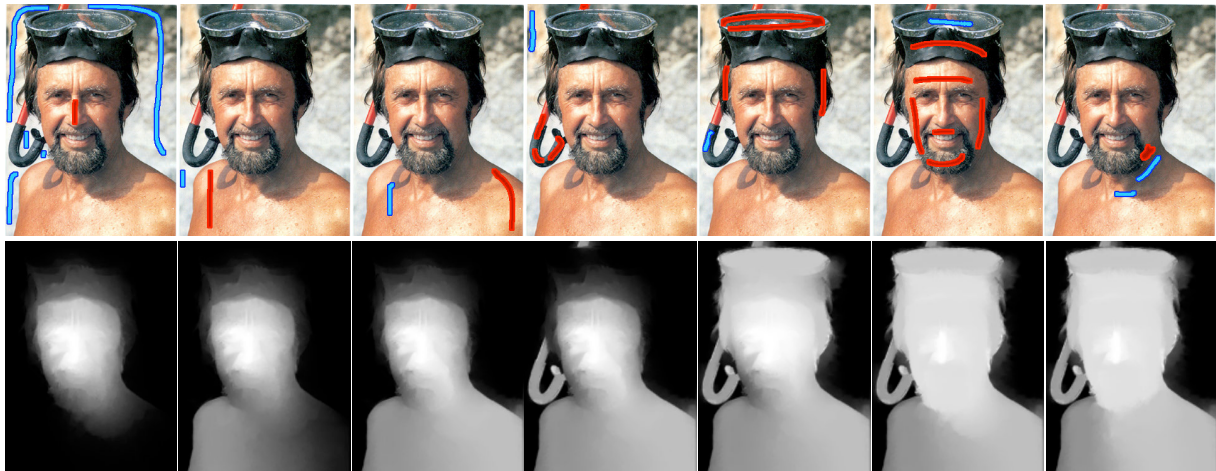
Figure 9: Top row shows the scribbles incrementally added by the user to differentiate the depth levels. A red scribble describes the image regions that should be closer to the camera. The bottom row shows how the depth map is updated after each pair of scribbles. Note how the relative constraints are incorporated at each step to change the depth map according to the user's needs. The scribbles are thickened for visualization clarity. Image by Michael Jung via Wikimedia Commons.
