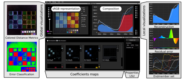
Figure 7: The graphical user interface, that focuses on several linked views: coefficients maps, global spectral error views and per-pixel views for detailed local investigations.
