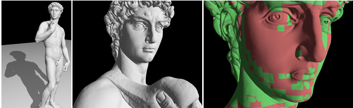
Figure 1: A 1 billion triangle model is rendered on a 1920 \times 1080 viewport using rasterization and ray-casting simultaneously. Ray-casting works on a sample-based surface LoD representation at an effective maximum sampling resolution of 8K^2 \times 32K . Red and green surface areas indicate parts of the model that are rendered via rasterization and ray-casting, respectively. On a GTX 680 graphics card the hybrid approach always renders the model in less than 30 ms ( > 33 fps) at a screen space error below pixel size.
