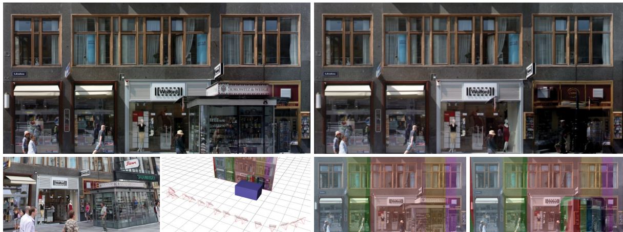
Figure 11: Top left: multi-view stitching without constraints. Top right: multi-view stitching with geometry constraints. Bottom from left to right: one of the original perspective shots, occluding geometry has been modeled into the scene, source-indication masks without and including the geometry occlusion.
