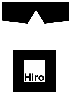
Figure 3: The experiments were made by printing the ARToolKit marker and the model of the polarization glasses to the same sheet of paper. As the transformation matrix between the markers is known, we were able to compare the results obtained by the two different tracking methods. The width of the polarization glasses was 12.6 cm and height 4.1 cm. The edge length of the ARToolKit marker was 8.0 cm. The origo was set to the center corner of the glasses.
