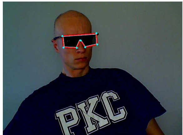
Figure 1: The edge of the front face of the polarization glasses is detected and its outer border is traversed (highlighted in red). The corner points of the polygon are detected to divide the edge into parts (cyan dots).
