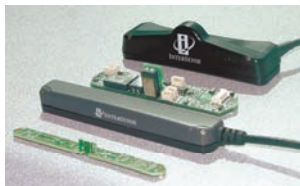
Fig. 2: Gen2 vs. Gen3 Head Tracker Circuits
