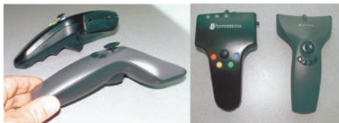
Fig. 1: Gen2 vs. Gen3 Wand Design
