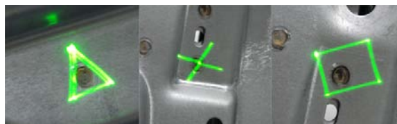
Figure 1: Different symbols projected on the welding points. Compare Fig. 3
