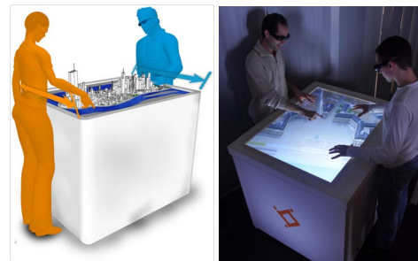
Figure 5: The concept (left) and the reality (right) of two users viewing a single 3D mockup and manipulating the 3D environment using dedicated interaction techniques.
