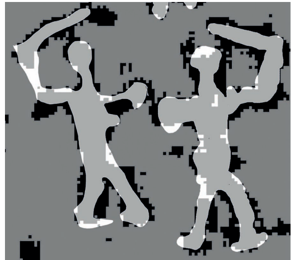
Figure 5: Segmentation results with the feature GLCM-Stat32 overlaid with the ground truth. Light gray pixels denote true positives, dark gray pixels true negatives, black pixels false positives and white pixels false negatives. Please note that the results are without any post processing.
