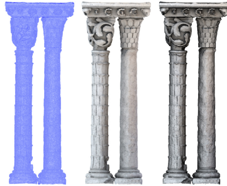
Figure 2: Column of the Abbey of Saint-Guilhem-le-désert. Visual levels (geometry, textures, occlusion + textures) [DDL08].
