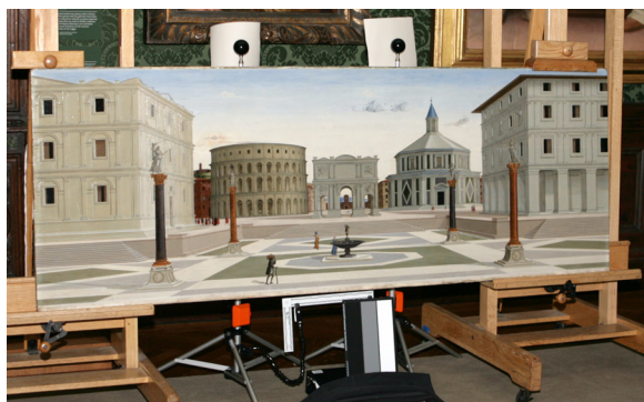
Figure 2: RTI set up for large panel painting: reference spheres at top, scale and color target below.
