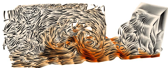
Figure 8: Streamlines depicted with tadpole-shaped, fixed size patterns, combined with a ‘halo’ colored using a colormap (velocity).
