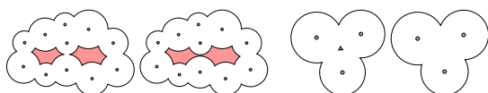
Figure 1: Left: Two cavities that are apparently very near to each other may be a single cavity. Right: A very small cavity may be reported whereas no such cavity may exist.
