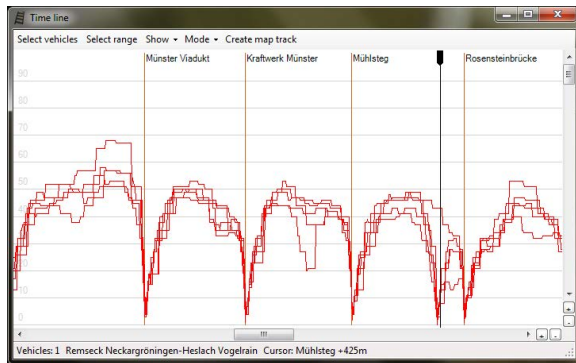
Figure 1: The diagram view displaying the vehicle speed during multiple trips of a single vehicle along the stations of a route (route pattern range).
