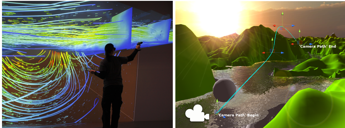
Figure 3: (left) Stereoscopic visualisation of an OpenFOAM and Min3P simulation [TSM*13] of stream flow in the hyporheic zone in a virtual reality environment. (Data kindly provided by N. Trauth), (right) Visualisation of the Rappbode reservoir in Unity3D, including camera paths and visual effects employed for interactive presentations.
