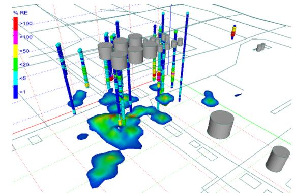
**Figure 3:** LNAPL plume (color blobs), LIF responses (tubes of color spheres), and former aboveground storage tanks (ASTs) at a former gas plant in the southwestern U.S.
