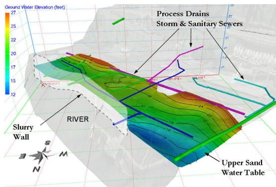
**Figure 2:** Potentiometric condition in an upper sand unit at a petroleum fuel terminal in the northwestern U.S. The transparent surface is the upland topography and river bathymetry.
