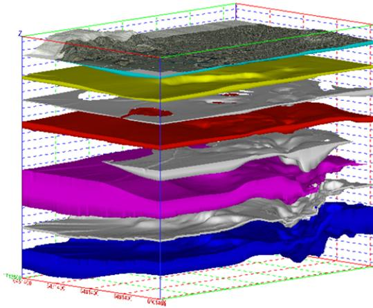
**Figure 1:** Stratigraphic units (exploded view) near a coastal area in the western U.S. An aerial photo of the region is shown on the top layer. The color structures are aquifers and the silver structures are aquitards.
