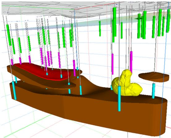
**Figure 4:** Chlorinated solvent DNAPL contamination (red layer and yellow blob) beneath an industrial facility in the northeastern U.S. The brown layers are aquitards and the color tubes represent the screen intervals of monitoring wells.
