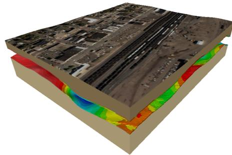
**Figure 5:** A two-unit structural model for a railroad site in the northern Midwest of the U.S. An aerial photo of the site was shown on the upper surface; the contact between the two units was illustrated as a series of colored iso-elevation contours.
