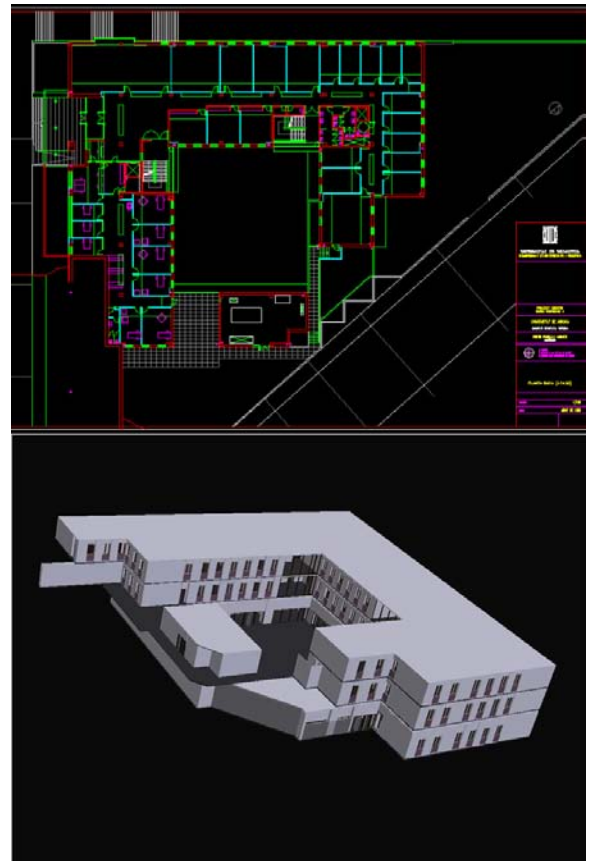
Figure 16: Above, the University of Girona P4 building 2D floorplan. Below, the 3D generated model
