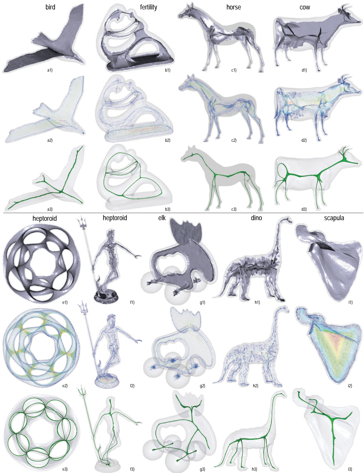
Figure 1: Examples: Medial surfaces (a1-i1); medial point clouds colored by importance (a2-i2); curve skeletons (a3-i3).
